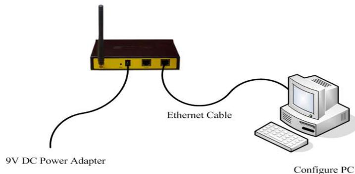
Please modify the IP address of PC as the same network segment address of the router, for instance, 192.168.1.9. Modify the mask code of PC as 255.255.255.0 and set the default gateway of PC as the router's IP address (192.168.1.2).
