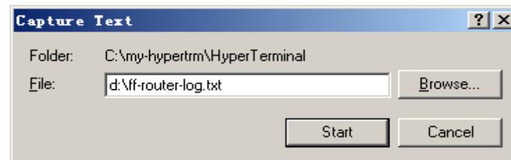
Input the log file name and press “start” button, the output message are now stored in the log file.
