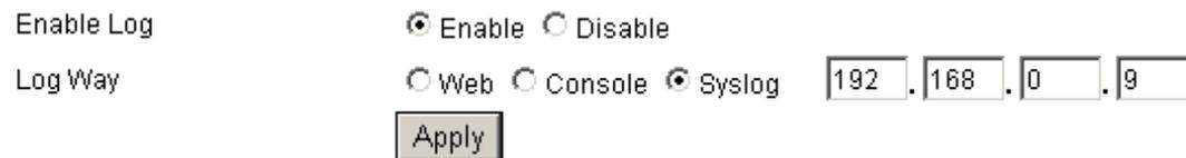
The log message is output to a syslog server, if choose this way, you should input a syslog server’s IP Address and run a syslog server program on it .
